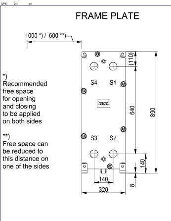
Space between pressure plate and supporting column should be kept free from fixed installations!
